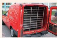
Example: shelf system in module construction, individually custom-fit to your vehicle. Manufactured on request
